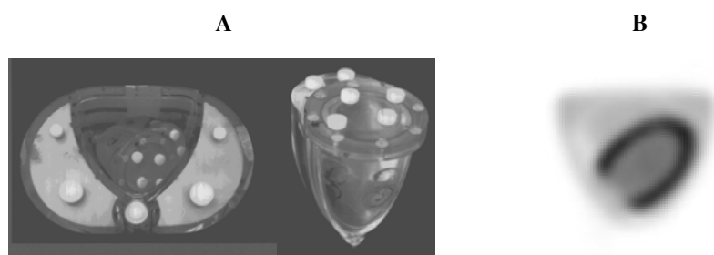
Figure 2. (A) Photograph of the heart/chest phantom and (B) typical reconstructed transaxial slice at the level of the myocardial wall.
